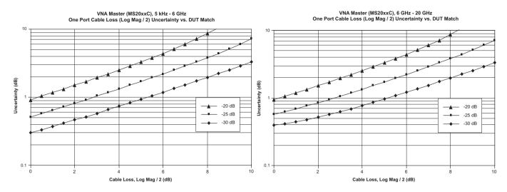
These uncertainty curves show how frequency range, DUT Match, and cable loss impact worst-case uncertainty of round-trip cable loss measurements. The uncertainty curves, separated by frequency range, are shown for DUT Match cable loss conditions of -20 dB, -25 dB, and -30 dB. For DUT Match of 30 dB and cable loss of 4 dB to 5 dB (reflection measurement of 8 dB to 10 dB) the worst-case uncertainties are approximately  $\pm$  1 dB.
