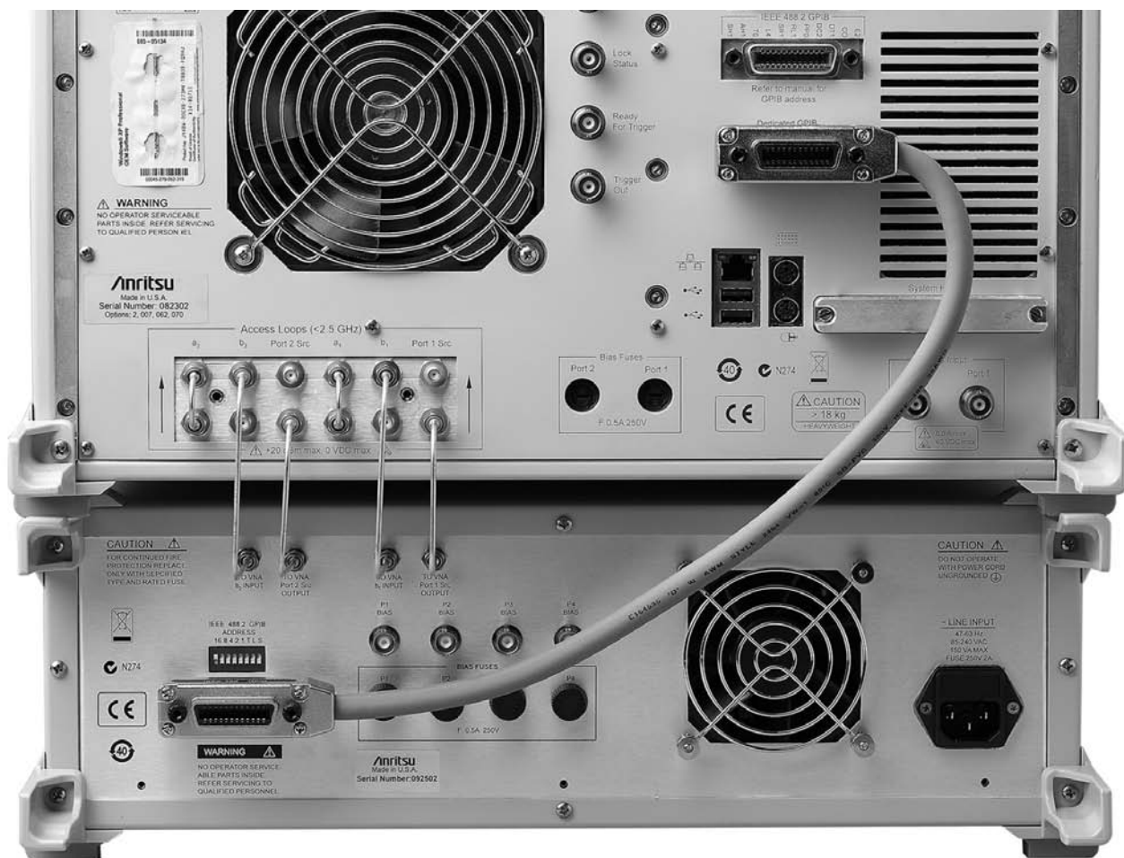
MN469xB Test Set Rear Panel and connections to base VNA.
