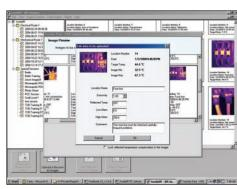
Assign a unique name, preset emissivity and RTC values, assign alarm limits and add meaningful comments to each measurement location.
