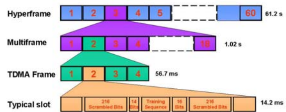
Figure 1 - Air Interface - TDMA illustrated
