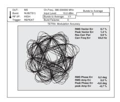
For diagnosing problems, EVM, phase and amplitude errors can be displayed as a graph against time.
